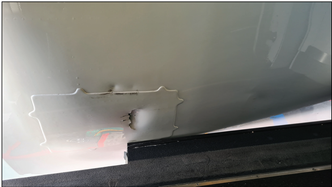
Photo 2. Damage to the aircraft fuselage skin.
